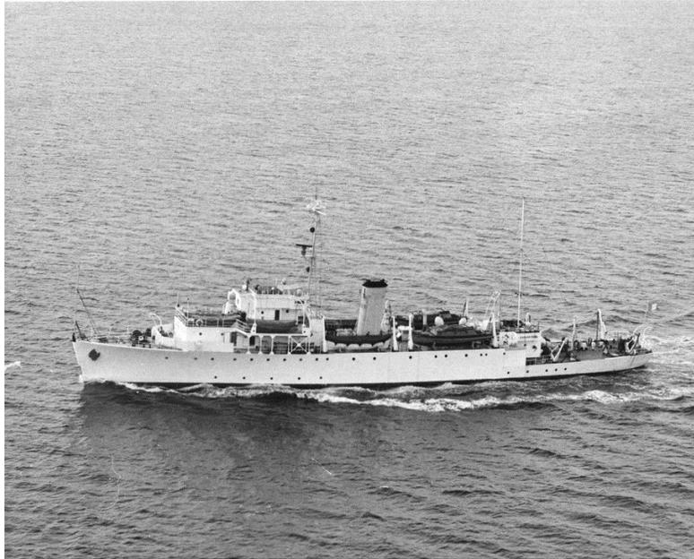
The CHS *Baffin* was a diesel-driven ship initially equipped for hydrographic surveying but later was also used for general oceanography. She was built in 1956 by Canadian Vickers in Montreal, QC, with a Lloyds Ice Class I hull to enable work in ice-infested waters. She was equipped with twin screws and a bow thruster. She was capable of carrying six hydrographic launches and a helicopter. At the time, she was the most modern hydrographic survey vessel in the world. Her vital statistics were:
