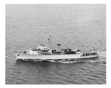
The CHS *Baffin* was a diesel-driven ship initially equipped for hydrographic surveying but later was also used for general oceanography. She was built in 1956 by Canadian Vickers in Montreal, QC, with a Lloyds Ice Class I hull to enable work in ice-infested waters. She was equipped with twin screws and a bow thruster. She was capable of carrying six hydrographic launches and a helicopter. At the time, she was the most modern hydrographic survey vessel in the world. Her vital statistics were:
