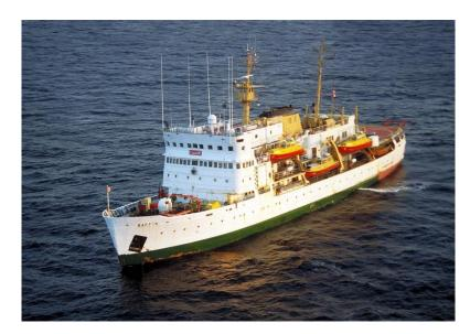
The CHS *Maxwell* was a diesel-driven ship built for inshore hydrographic surveys. She was designed by German Milne and built at Halifax Shipyards in 1960. She was delivered in 1961 and capable of carrying two hydrographic launches. Her vital statistics were:
