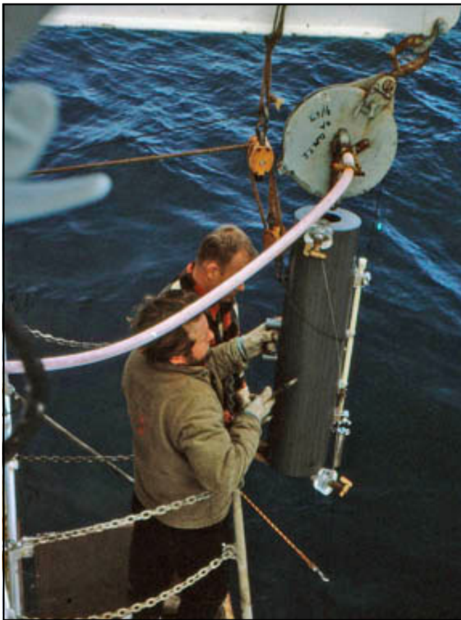
Roger Pocklington and Bob Cooke putting a 30-litre Niskin sampling bottle on the wire.
