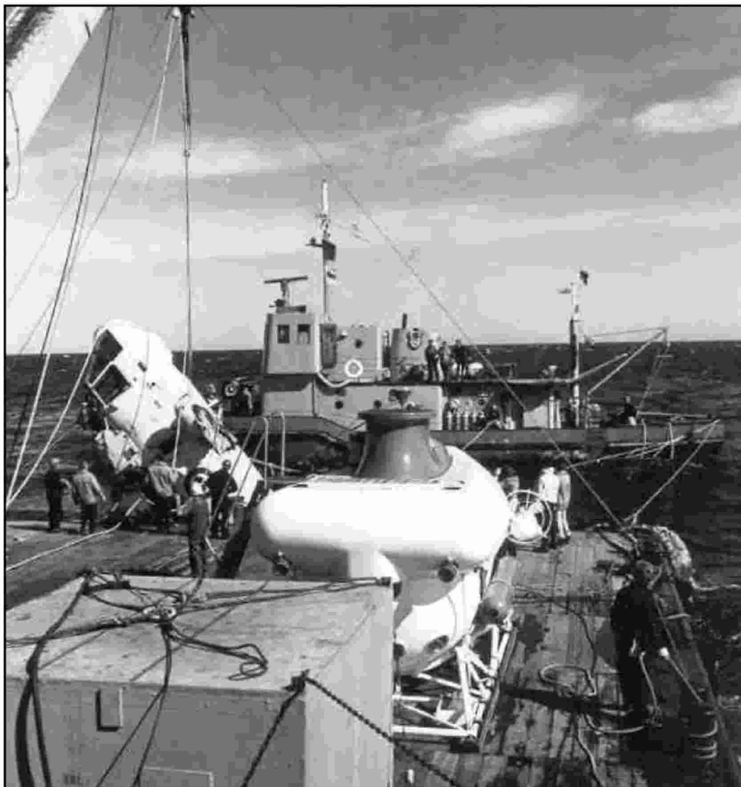
The Sea King helicopter is winched aboard a barge after its recovery by the SDL-1 submersible (foreground). Photo courtesy of the Canadian Forces.
