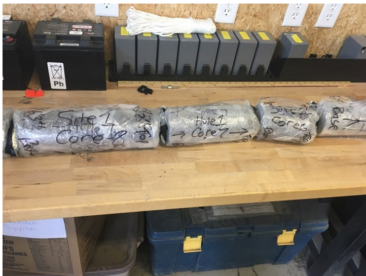
Fig.3 Permafrost core samples taken from Tuktoyaktuk Island required quick analysis to avoid thawing while out of the freezer.
