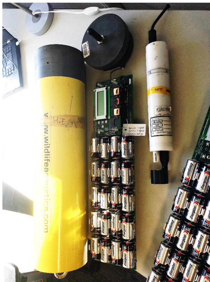
Fig. 2) The yellow casing and song board with all the D cell batteries attached to it is one of five hydrophones which I've programmed. The white cylinder is one of six instrument loggers which I've programmed, in this case we have a Conductivity Temperature Depth (CTD) logger.
