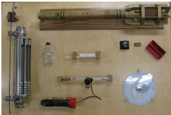
Fig. 1 - Tools of the trade for physical oceanography in the early 1960s. From the top: bathythermograph (BT) for measuring water temperature at various depths; slide holder and glass magnifier for reading slides from the BT; special slide rule for converting thermometer readings to temperature and depth; illuminated magnifier for reading reversing thermometers; just above is a reversing thermometer; above that is a standard sample of sea water used to compare recovered samples; to its left is a sterile water bottle for storing seawater samples for later testing; far left is a Knudsen water bottle for collecting seawater samples. (Photo courtesy of BIO OA website)
