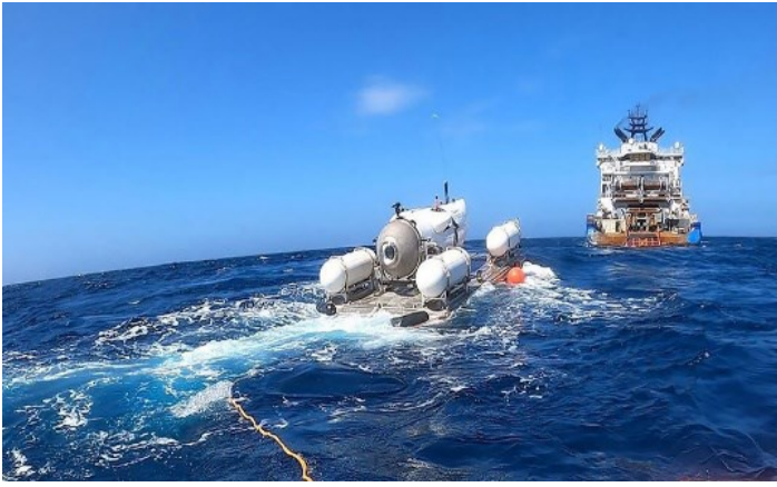
Figure 2: OceanGate Expeditions Titan onboard platform in tow by tender vessel for deployment/recovery at the RMS Titanic wreck site in the North Atlantic 650km southeast St John's, Newfoundland. Source: OceanGate Expeditions
