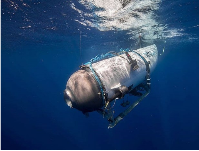
Figure 1. OceanGate Expeditions 6.7m long, 10,500 kg Titan manned submersible descending below sea surface. Source: OceanGate Expeditions
